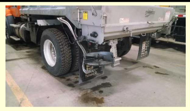
BEET HEET® is pumped from a storage tank to the back of the truck and sprays out of either one or two nozzles onto the salt right before the salt is applied to the roads.
