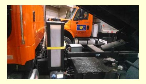
Each truck is equipped with either an 80 gallon underbody mounted tank or 100 gallon behind cab mounted tank.
