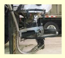
Spray nozzles Depending on the truck, each system will either have one or two nozzles. The size of the nozzles also varies between trucks from size 3 or 4.
