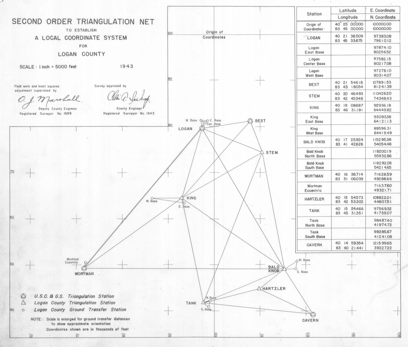
A complete description of each station used in the triangulation net is included in these pages. The first four stations, Wortman, Logan, Best, and Cavern, were described by the U. S. C. & G. S. The remaining stations are those established for the Logan County triangulation net and they were described by the thesis group.
