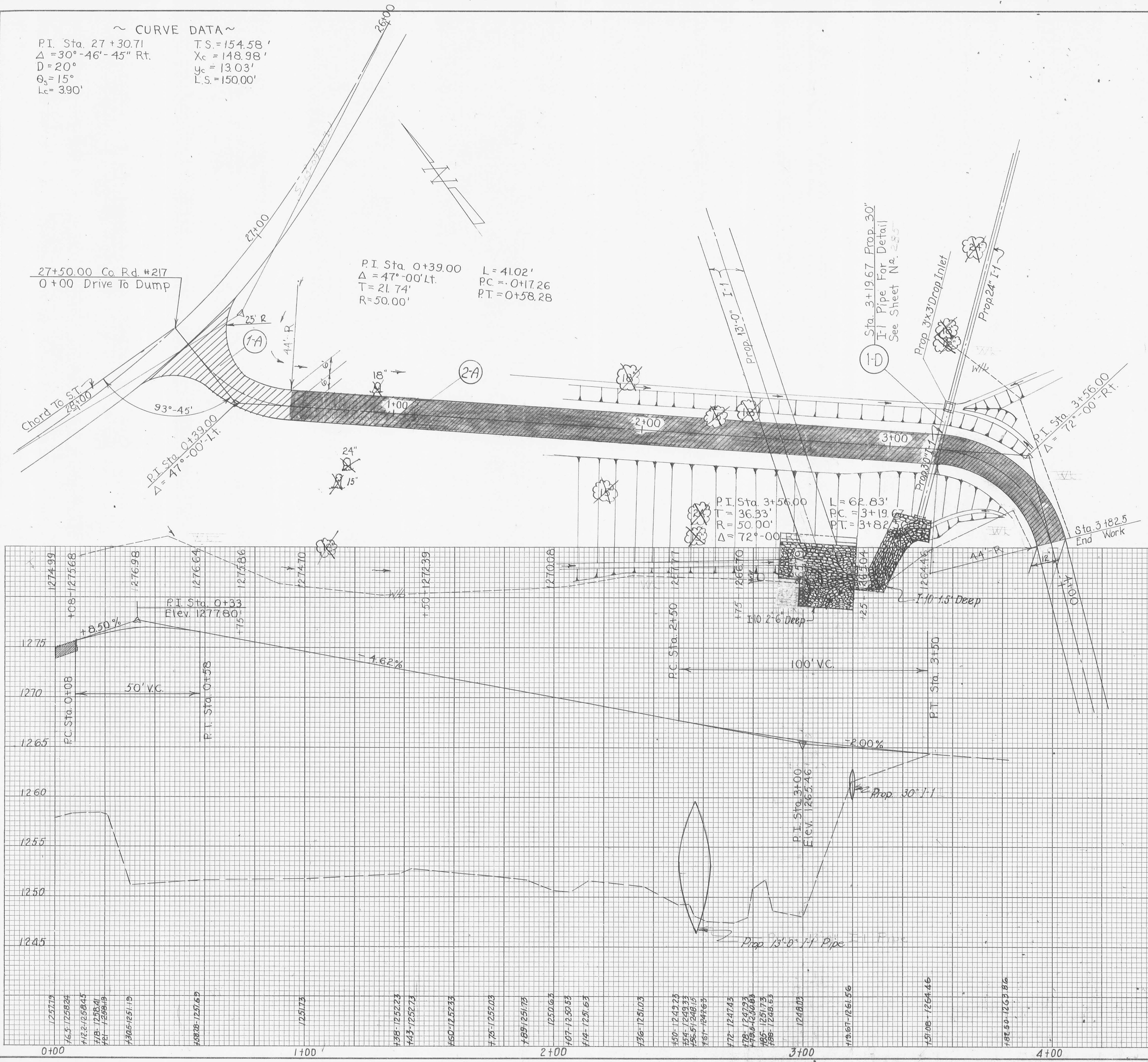
PLAN & PROFILE STA. 0+00 TO STA. 4+00 DRIVE TO DUMP COUNTY ROAD # 217
