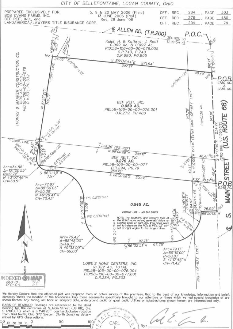
40 30 20 10 0 50 GRAPHIC SCALE: 1"=50 SURVEY MONUMENTS: Found (F)=0, Set (S)=0. IP=Iron Pipe (ID); SP=Solid Pin (OD); RB=Rebar; RS=Railroad Spike; MN=Mag Nail; PK=PK Nail & IPS=3/4"ID iron pipe set flush with the ground & capped with a yellow plastic plug inscribed C. TURNER/P.S. 6702.
