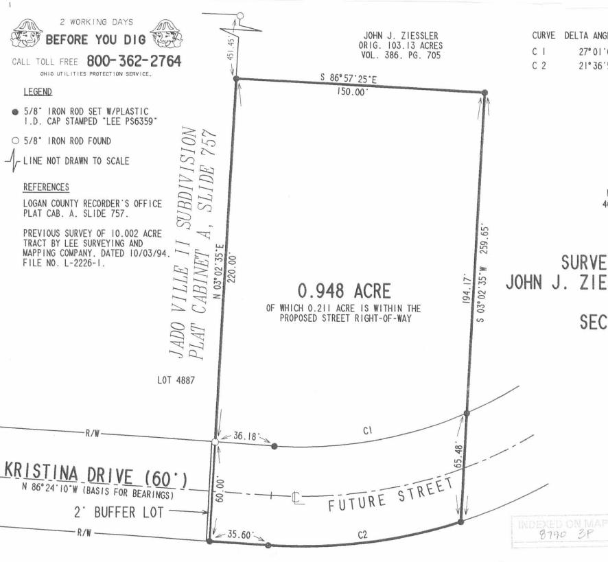
CURVE DELTA ANGLE RADIUS ARC TANGENT CHORD CHORD BEARING 27° 01'00' 250.00 117.88 60.06 116.79 S 80°05'20'W 21° 36' 56' 59.18 310.00 116.95 116.26 S 82° 47' 22° W
