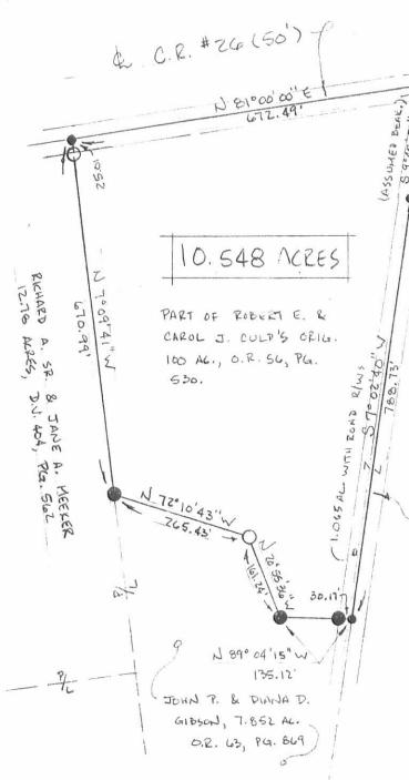
5/8" IRON PIN SET WITH CAP MARKED "CLAPSADDLE RS 6140"
