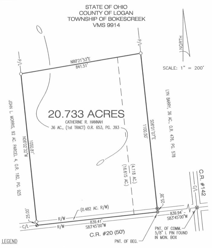
O - 5/8 " X 30" IRON PIN SET WITH CAP MARKED "GUIDER S 7752"
