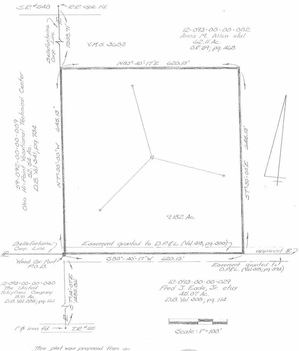
This plat was prepared from an actual field survey performed by the Logan County Engineer's Office. All angles and distances were measured in the field. Field work completed in June 1993.
