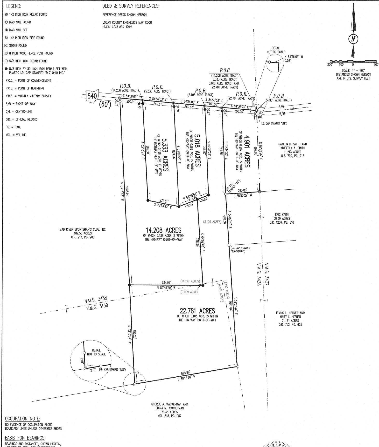
BEARINGS AND DISTANCES, SHOWN HEREON, ARE DERIVED FROM GPS OBSERVATIONS BASED ON GRID NORTH, OHIO STATE PLANE COORDINATE SYSTEM, NORTH ZONE, NAD83 (2011, EPOCH 2010), WITH THE CENTER-LINE OF OHIO ROUTE 540, HAVING A BEARING OF S 84'56'03" E.
