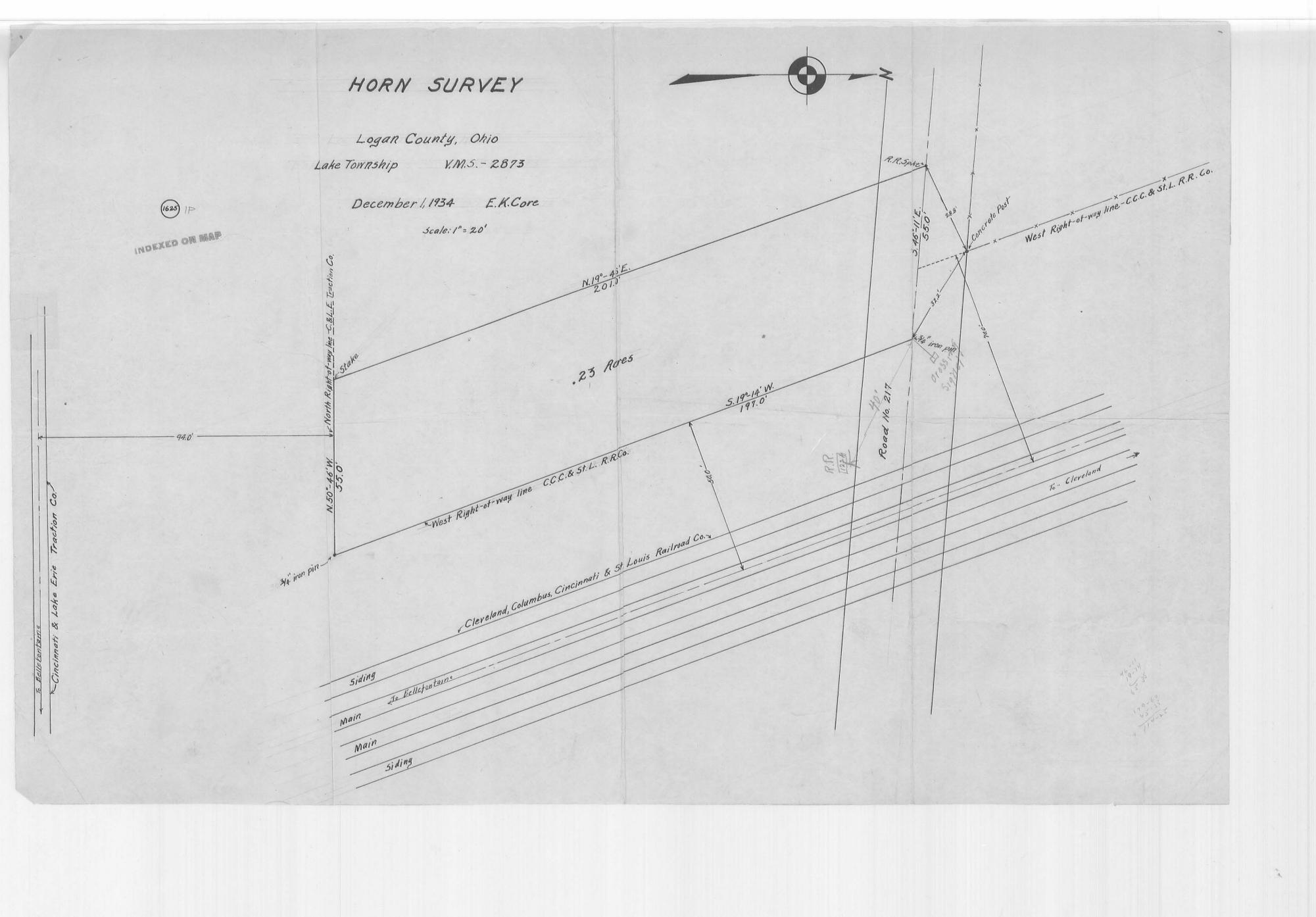
6-11-09 26 Horn Surv. N. of Bellef. Start - 905 pipe, cent, road NE & of Fract of Z.62 a. surveyed by C.M.R. - with E. line said 262 a S2014W, 512 to state, in N. line rt-of-way Ohio Elec. Co. - with rt-of-way N 44W 131 (2m) N 50/2W; 1.66 to E. Time 17-of-- with Big 4 rt-of-way NZO1/4E 3.82 to iron spike, cent. public road . Wit: - 40" Lynn 5101/2W, 75 1/5 - with soid road 5 4814 E, 1.10 ch. to 1" 905 pipe, Wit: 14" Wal 5841/2 66/2 1/15-- 5 89 E. 1.86 to begin
