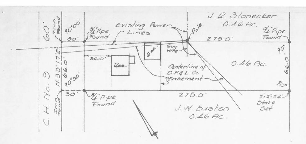
ROSTOFER SURVEY V.M.S. 3317 LAKE TOWNSHIP LOGAN COUNTY, OHIO JULY 8,1968 SCALE 1"=40' I hereby certify that this plat is a correct representation of a survey made by me and that the same shows the improvements as located on the premises.
