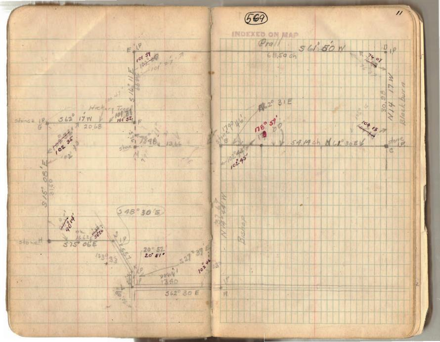
W. H. Montgomery John Herring Sponsler chicarriers ch carries Ocompor Survey Survey 2997 Nov 17- 1925 H, stone found Stone tound Auto Axle Driven point in O Cement Road Iron pin a 2' East of East Edge of Pau. Iron pin driven & East of Eastedge is Fence Post to tone found. Cor. Post · Pipe found on line with A + 0 71/o way See Drawing R Survey (988) 51839 10°W
