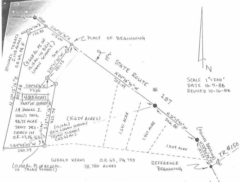
REFERENCE DEEDS SHOWN ON PLAT BEARINGS SHOWN HEREON ARE BASED ON AN ASSUMED. MERIDIAN AND ARE USED TO DENOTE ANGLES ONLY.
