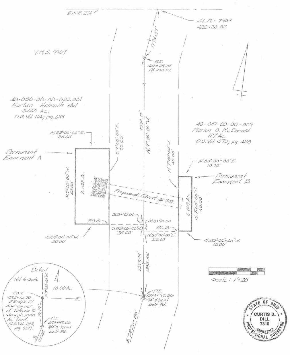
Basis of bearing being the centerline of Logan County Road No. 25 (N.7º00-00"W.) as shown on a 1990 Lee Survey of Harlan Helmuth's 3.000 acre tract (Index No. 5418).
