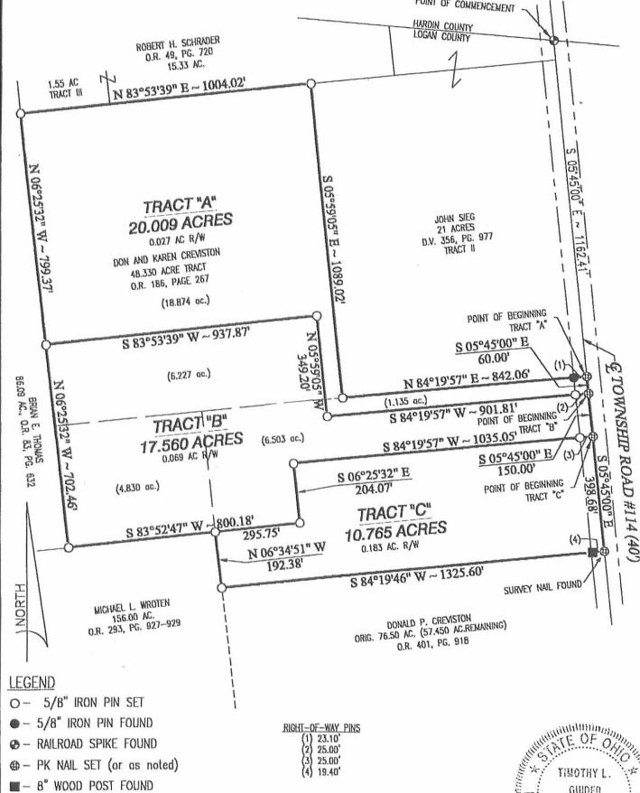
RIGHT-OF-WAYS SHOWN NOT TO SCALE FOR CLARITY BASIS OF BEARINGS C/L T.R.#114 FROM SURVEY BY LESLIE H. GEESLIN, 3/29/93 S05'45'00"E SCALE: 1" = 300'
