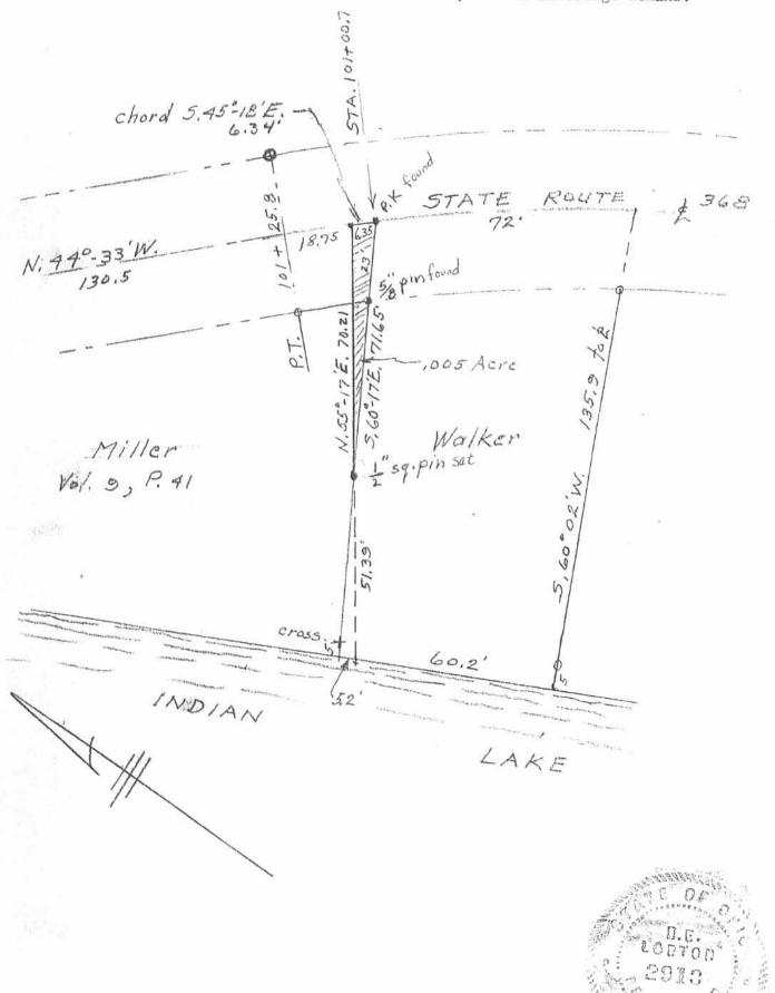
Bearing on State Route used as basis of bearing for this
