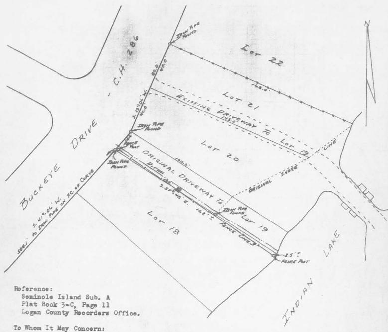
The above plat shows the line between Lot No. 18 and the Original 20.0 foot driveway to Lot No. 19. The existing fence does not follow this line. The fence on the West end is 0.5 of a fost north of the line. The fence on the east end near the waters edge in 2.5 feet south of said line. Iron pipes found as noted on Plat.
