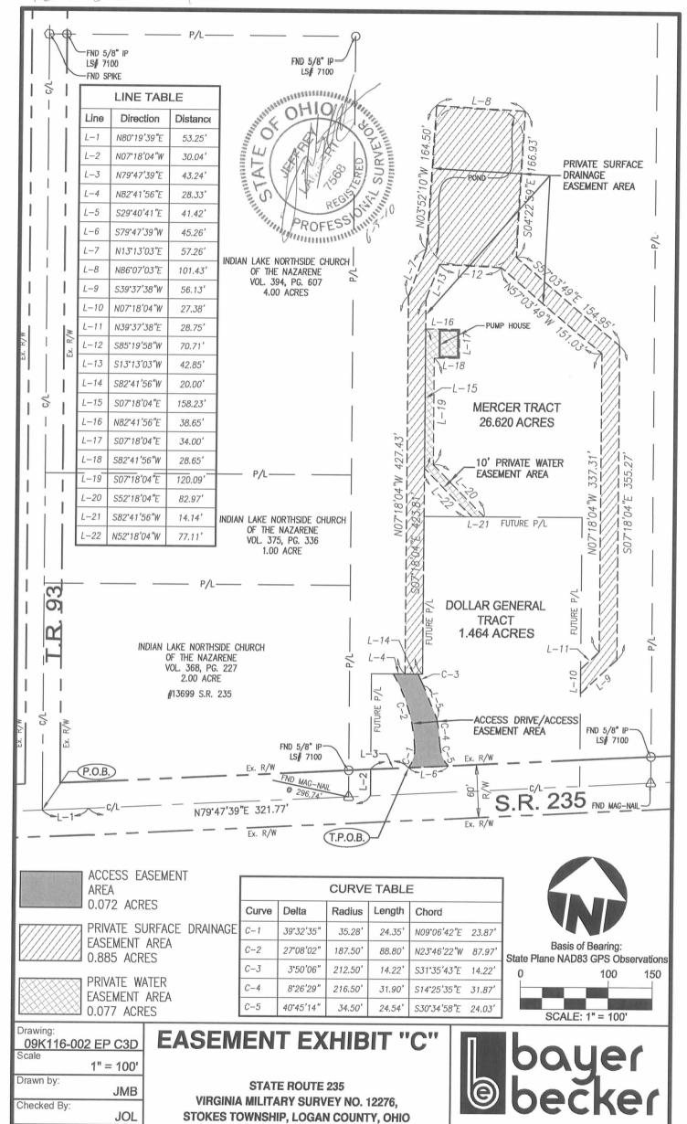
6-3-2010 ACCESS, WATERLINE, & STORM DRAINAGE EASEMENT
