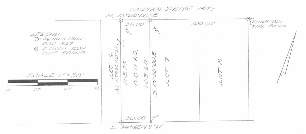
SURVEY OF A 30' STRIP ON THE EAST SIDE OF LOT 6 OF BERGS ALKOT. IN WASHINGTON TOWNSHIP, LOGAN COUNTY, OHIO AS PECORDED 'N THE LOGAN COUNTY RECORDER'S PLAT CABINET"A" SLIDE 164 "OF RICK ARCHER JUNE 18, 1992
