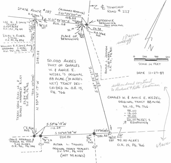
REFERENCE DEEDS SHOWN ON PLAT REFERENCE LOGAN COUNTY ENGINEER SURVEY . F.B. 558 , PG. 46-49 BEARINGS SHOWN HEREON ARE BASED ON AN ASSUMED MERIDIAN AND ARE USED TO DENOTE ANGLES ONLY.
