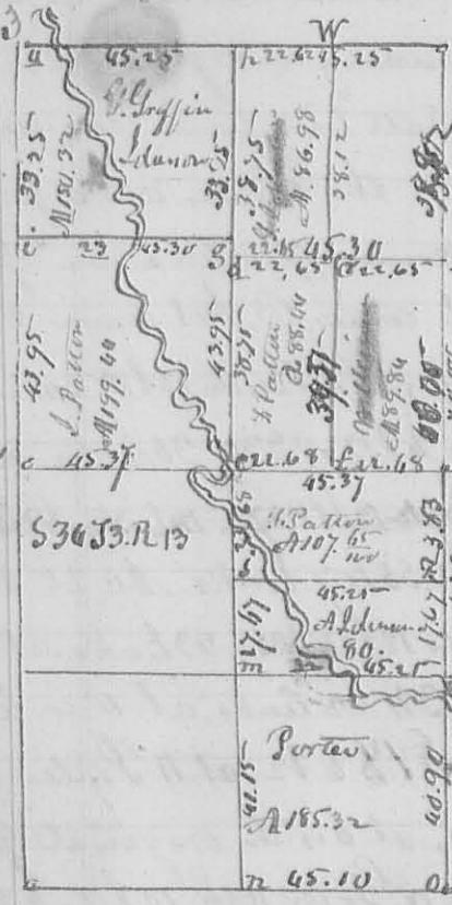
This plat represents the Survey & Sat. division of S35 T. 3 R 13 U. R. S. Original bearing of the lines due course by the Comr. prop. present variation  $^{\circ} E$ . the length of the lines marked on the plat, together with the N. of Acres, the figures with - under them, show the curving of Indian Creek, which passes through them.
