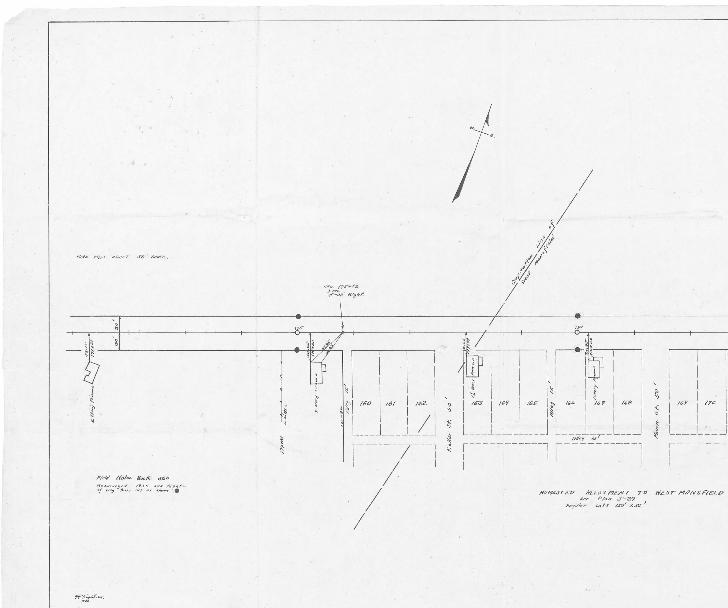
ROAD NO. 8 PERRY & BOKESCREEK TOWNSHIP 4 LOG AN COUNTY 4 1933 Length 18527 Feet (To curb) Length 3.5090 Miles (To curb) Length 3.3778 Miles (To corporation Line) 185 -0-16.40 To Face - Curb an gutter 3 Stone Walk End of Curb Sta. 185127 End of Walk sta. 1851275 173 174 170 171 172 1 (1376) INDEXED ON MAP x-8B
